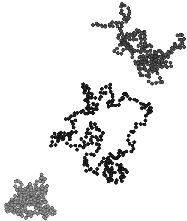
FIG. 2. Configurational snapshots of rings of mass N=256 : dilute flexible ring in the middle, flexible ( \sigma=0 ) ring in the melt ( \phi=0.5 ) on the left, and corresponding semiflexible ( \sigma=3 ) coil on the right. The overlap has increased by factor 3 between the flexible and semiflexible chains in the melt. To obtain a similar effect by increasing the chain mass we would have to increase N by at least two orders of magnitude.
